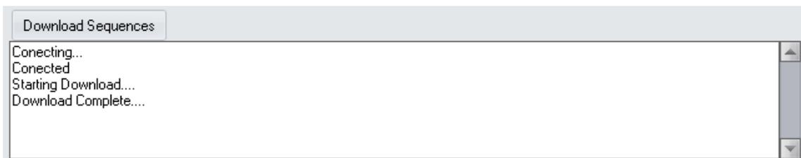
This plug-in download procedure requires a previous individual address assignment to the device. If the DM480330 has a different individual address, has no address assigned or the ETS cannot to it due to any other reason, the plug-in application will show a failure and the sequences will not be downloaded.
